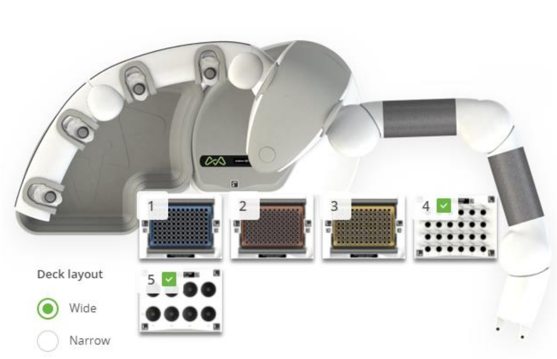
Figure 2 Andrew+ deck configuration for the triptorelin working solutions preparation protocol.
